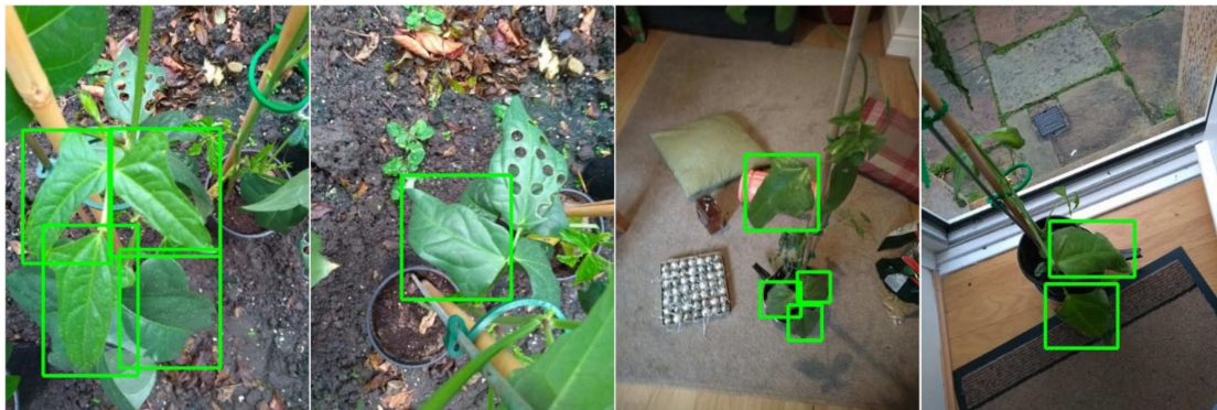
Figure 5. Four example pictures used for training the neural network. Leaves were only selected if they were not occluded or cropped—the method for estimating position is reliant on full leaves being labelled by the classifier.
