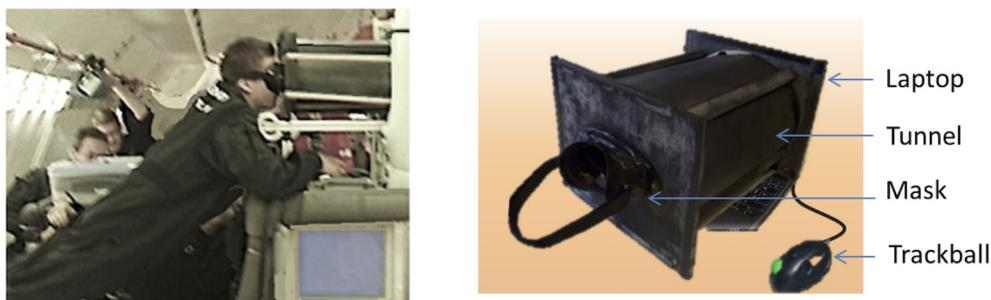
**Fig 2. The measurement device.** The measurement device consisted of a laptop mated with a tunnel and a diving mask. Participants looked at the visual scene displayed onto the screen. The visual scene was a picture of a room in which a doorway-like aperture was formed between two movable partitions. Perceptual adjustments were performed using a right-handed trackball.
