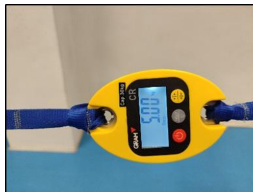
Figure 2. Image of the dynamometer showing 5 kg of lateral force generated by the elastic band on a participant.
