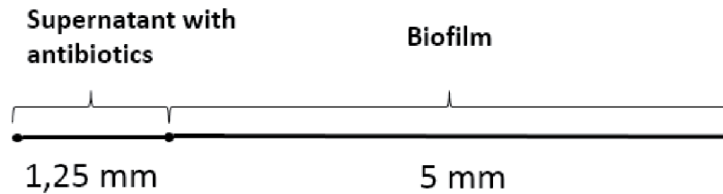
Fig 3. Geometry of ciprofloxacin model coupled with oxygen treatment. Sketch of the 1-dimensional model implemented in MATLAB. The origin is placed at the interface between the supernatant and the biofilm domains, hence the top of the supernatant has coordinate z = -1.25 mm, the top of the biofilm has z = 0 mm, and the bottom of the biofilm has coordinate z = 5 mm.
