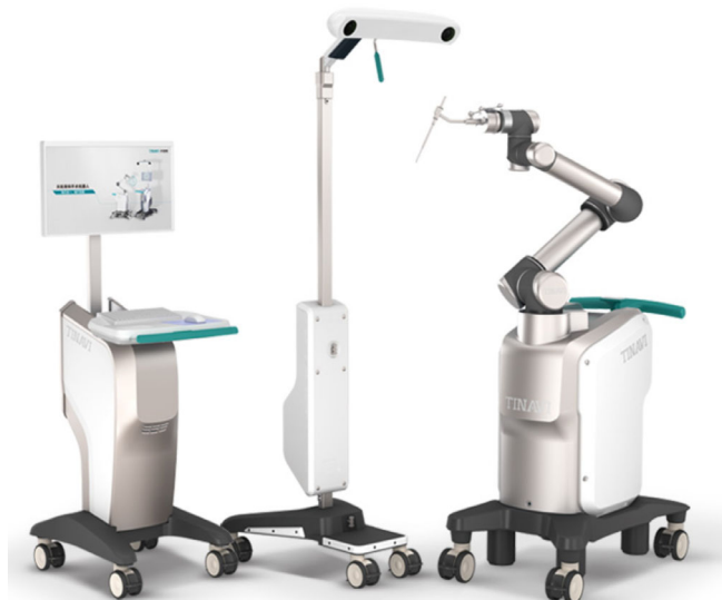
Fig. 1 The “TiRobot” orthopaedic robot, developed by TINAVI Medical Technologies, provides a new technology that facilitates the precise placement of pedicle screws. Main components of the TiRobot: robot arm, optical tracking device, surgical planning, and control workstation.
