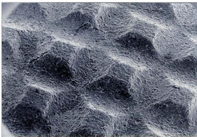
Figure 5 SEM Image of the surface of a removed cup.
