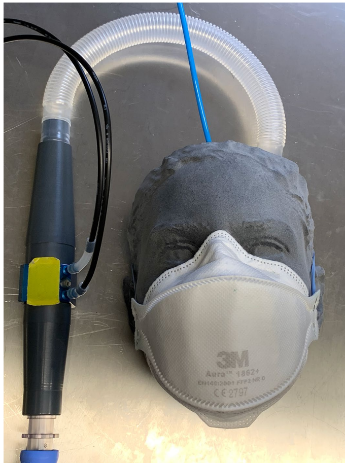
Figure 9. Measurement setup for the FFP2 mask while simulating human-like breathing. The pressure tubes exiting the obstruction flow meter (black) and the tube coming from the inside of the mask (blue) are connected to a pressure sensor array.
