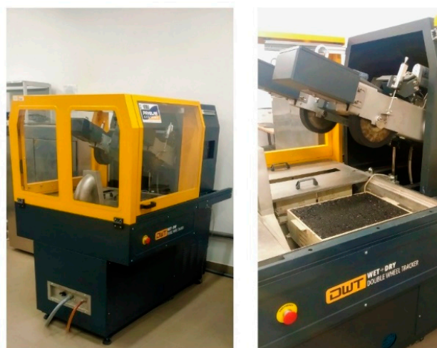
Figure 2. DWT test device and sample setup.
