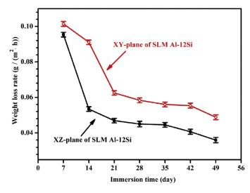
**Figure 7.** The weight loss rate for the different surface planes (parallel to the building platform—XY—and perpendicular to the building platform—XZ) of as-built and mechanically polished SLM AlSi12 after immersion in 3.5 wt.% NaCl solution at room temperature [42].
