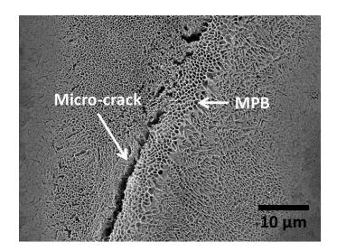
**Figure 2.** Secondary electron microscopy image of the surface of an as-built additive manufacturing (AM) Al-Si (AlSi10Mg) after immersion for 48 h in 0.1 M NaCl. The formation of micro-cracks in the heat affected zone next to the MPB can be seen. MPB—melt pool border.
