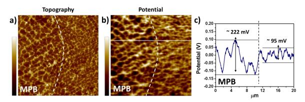
**Figure 5.** (a) Topography and (b) surface potential map (obtained by scanning Kelvin probe force microscopy—SKPFM) of an area on the surface of a polished AM AlSi10Mg specimen in which a melt pool border is visible (delimited by the discontinuous line). Scan size:  $20 \times 20 \ \mu\text{m}^2$ . Colour bar: (a) 30 nm range, (b) 210 mV range. (c) Surface potential profile of the line represented in (b). (Adapted from reference [32]).
