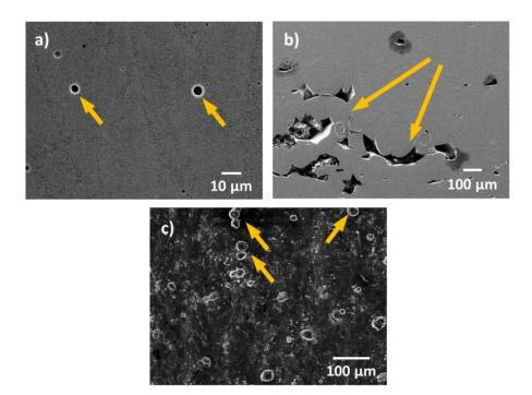
**Figure 1.** Secondary electron image representing defects that can be present in additively manufactured metal parts: (**a**) trapped-gas pores; (**b**) lack-of-fusion pores; (**c**) unmolten powder.
