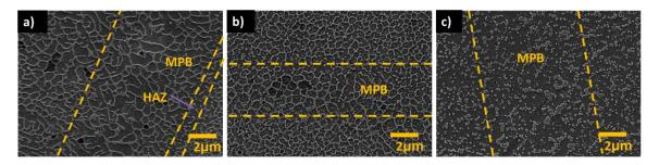
**Figure 8.** Secondary electron image showing the microstructure of (**a**) an as-built AM Al-Si sample (AlSi10Mg), as well as two stress-released specimens: one at 250 °C for 2 h (**b**), and another at 300 °C for 2 h (**c**). MPB refers to the melt pool border, while HAZ stands for the heat-affected zone. (Adapted from reference [54]).
