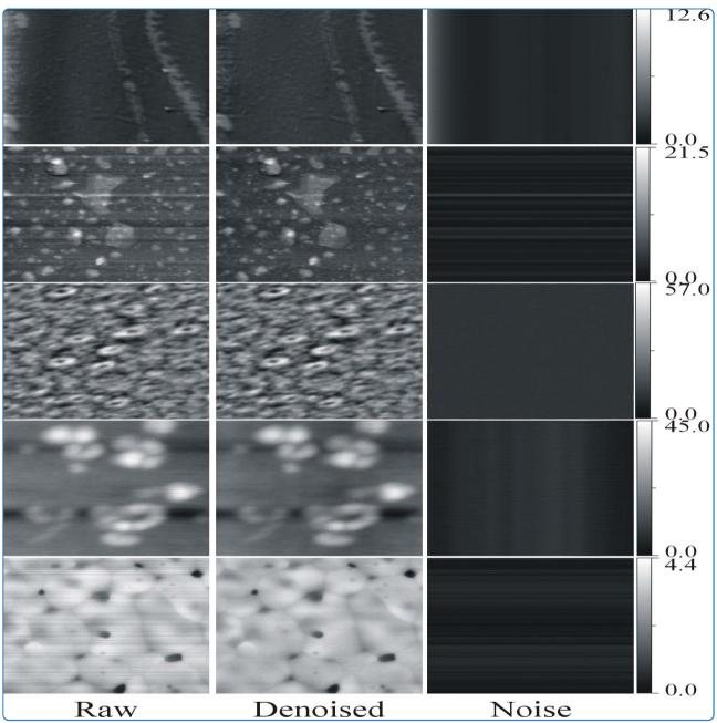
DeStripe: frequency-based algorithm for removing stripe noises from AFM images
