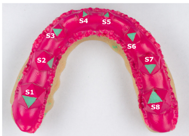
Figure 2. Example splint after “grinding surface” preparation and powder spraying. S1 to S8 depict the respective grinding surfaces.
