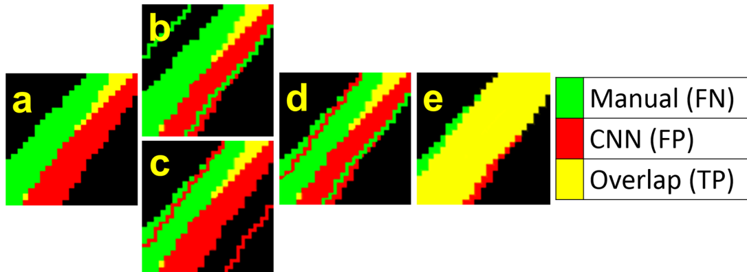
Figure 4. A modified Dice coefficient accounts for slight spatial differences between manual ground-truth and CNN segmentations of the same capillary. (a) Example in which manual (green) and CNN (red) segmentations of the same capillary have little overlap (yellow), yielding a very low Dice coefficient of 0.14. (b) To account for slight spatial differences in segmentations of the same capillary on measures of performance, the boundaries of the ground-truth segmentation were expanded outward by 5 pixels (green lines). (c) The boundaries of the CNN segmentation were expanded outward by 5 pixels (red lines). (d) Image showing the upper and lower boundaries of the intersection of the two expansions from (b) and (c). The pixels within these boundaries are considered to be overlapping pixels, or true positives. (e) The new overlapping region (yellow) was used to calculate the modified Dice coefficient (with a value of 0.93 for this image).
