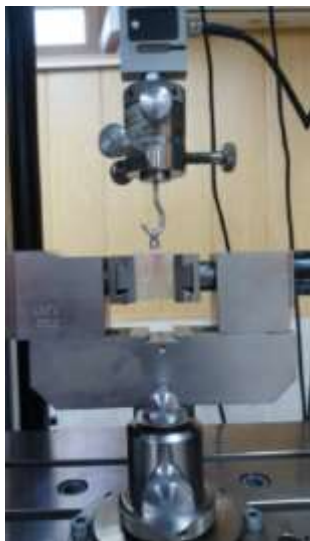
Fig 1. Tensile test to measure the retention of copings
