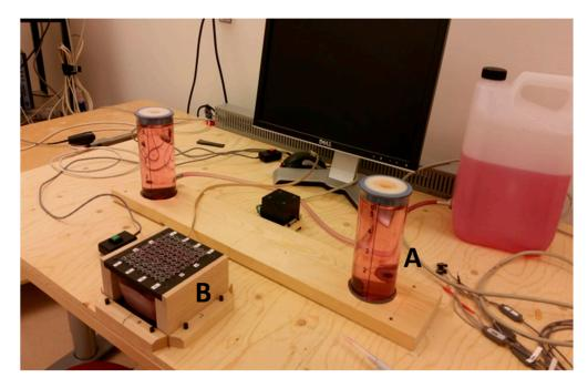
**Figure 2.** Arrangement of target and pickup tubes; the right, larger tube (A) was the pickup tube, and liquid was to be dispensed into small tubes in the fixture at the front (B).
