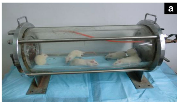
Fig. 2 A The hypobaric hypoxic chamber model. B Schematic of the hypobaric hypoxic chamber. (a) Closed chamber (radius, 15 cm; length, 65 cm); (b) rat access channel; (c) air inlet valves; (d) manometer (range, 0–760 Torr); and (e) vacuum pump. Twelve rats were placed in the closed
