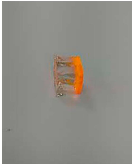
**Figure 5.** icPad of length  $10 \times$  width  $10 \times$  depth  $4 \text{ mm}^3$  was cut for extraction of fluorescence dye.
