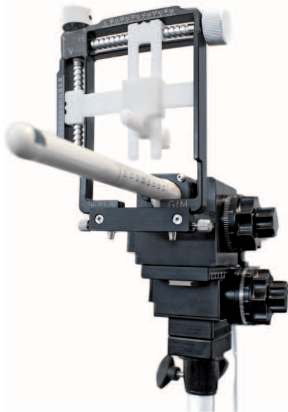
Fig. 2. The one-hole needle guidance device
