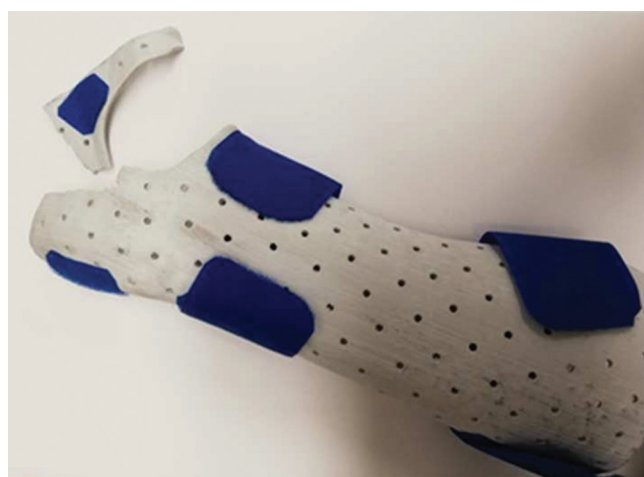
Figure 5. Partial breakage of a 3D wrist immobilizing splint.
