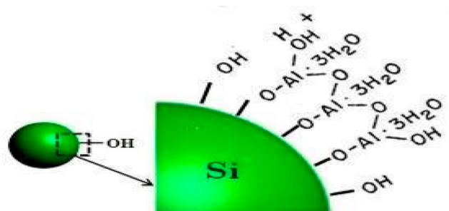
Figure 6. Sketch of the silica-coated nanoparticles with alumina on a modified surface. 62
