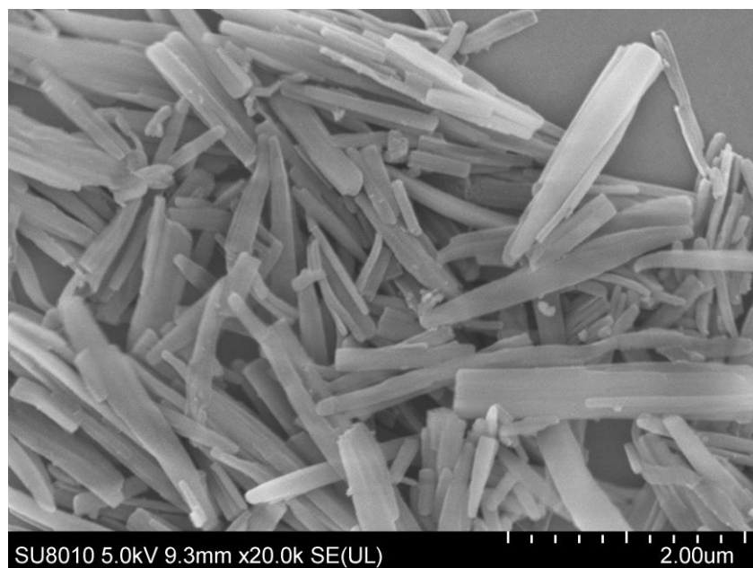
Supplementary Fig. 8 | SEM image of Py-DAB.
