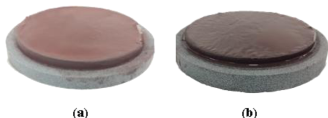
Figure 12. Filter-cake with (a) 100% hematite and (b) 25% ilmenite.
