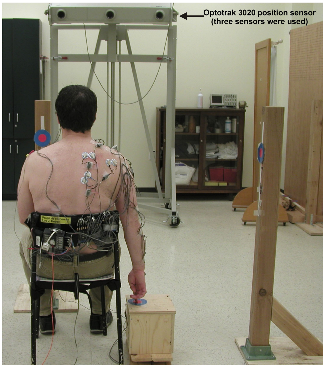
Figure 1 Starting position for the reaching movement. The reaching movements started with the upper extremity in a neutral position at the side of the body and the tip of the second finger in contact with a pressure switch. The kinematic was characterized using an optoelectric system and infrared light-emitting diodes positioned on five upper limb landmarks. As seen on the Figure, electromyography activity was also recorded, but the data were not analyzed in this study.
