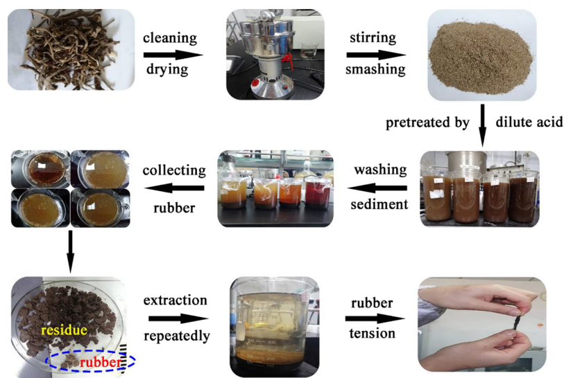
Figure 1. Pretreatment experiment operation steps.
