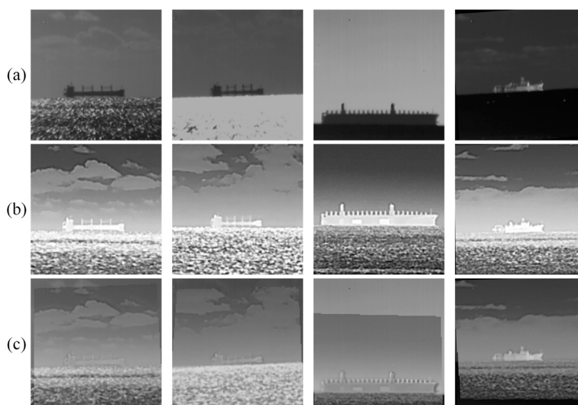
Fig. 9. Partial infrared images of ships in multiple bands. (a) SWIR, (b) LWIR and (c) Fusion of SWIR and LWIR.
