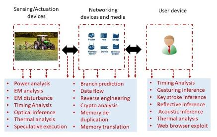
Figure 2. Side-channel attacks for a typical digital agriculture application.
