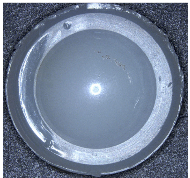
Fig. 5. Burnishing observed on the dome of the polyethylene component of a retrieved total disc replacement.
