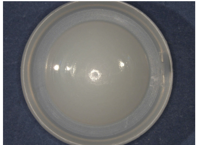
Fig. 18. Charité components tested using ISO wear testing protocols incorporating coupled motions exhibited regional burnishing and wear at a rate of 0.124 mm/Mcycles.
