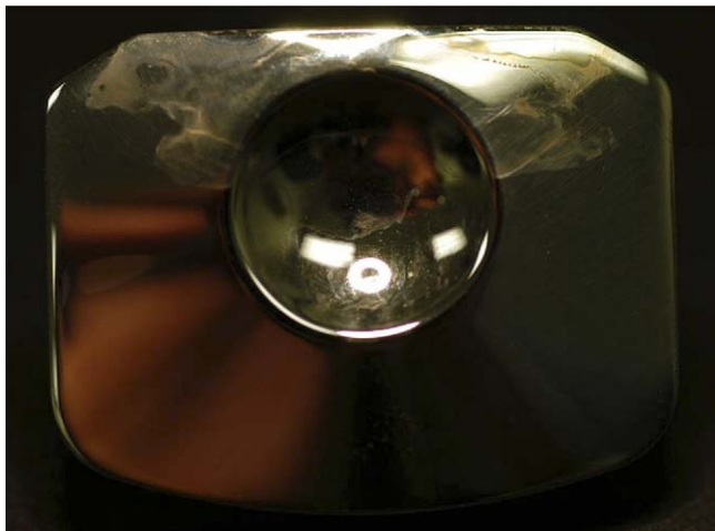
Fig. 12. Biofilm observed in CoCr alloy, metal-on-metal total disc replacement.
