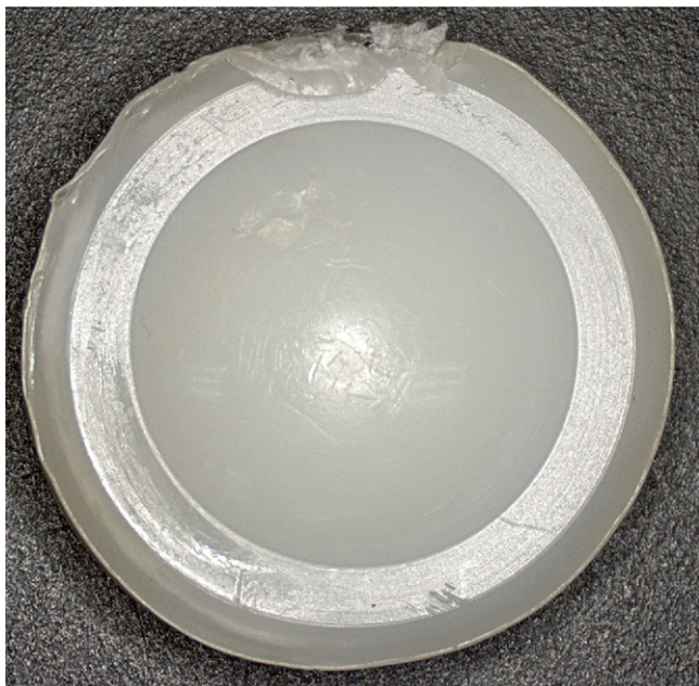
Fig. 4. Microscopic, multidirectional scratches and crisscrossing wear paths at the dome of a retrieved polyethylene total disc replacement that was implanted 6.2 years.
