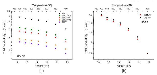
Figure 5. Total conductivity plots as a function of temperature for (a) BCFZY<sub>X</sub> series and (b) BCFY under wet and dry atmospheres.
