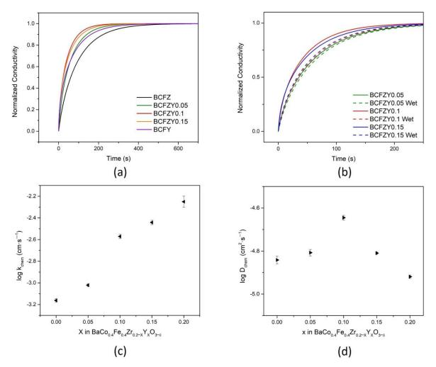
**Figure 6.** Electrical conductivity relaxation curves at 600 °C. For (a) BCFZY<sub>X</sub> samples and (b) BCFZY0.05, BCFZY0.1, and BCFZY0.15 under wet and dry atmospheres; the fitted dry atmosphere curves yield the (c) surface exchange coefficient,  $k_{chem}$ , and (d) bulk diffusion coefficient,  $D_{chem}$ .
