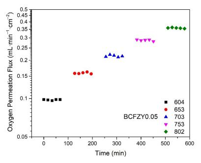
**Figure 2.** Oxygen permeation flux as a function of measurement time at increasing temperatures for BCFZY0.05, showing stable flux over each one-hour measurement.
