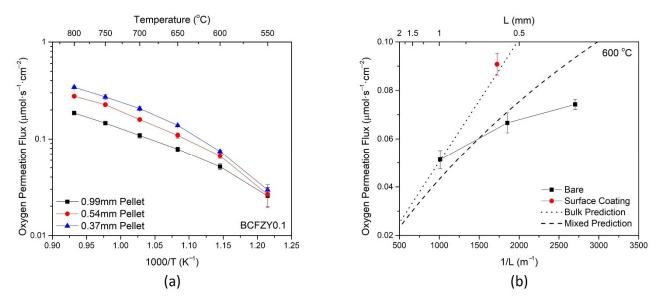
**Figure 4.** Oxygen permeation flux for the BCFZY0.1 sample (**a**) as a function of temperature, under varying thicknesses, and (**b**) as a function of thickness at 600 °C.
