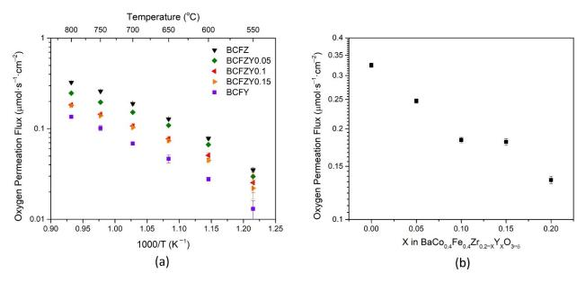
**Figure 3.** Oxygen permeation flux normalized for 1 mm BCFZY<sub>X</sub> pellets as a function of (**a**) temperature, and (**b**) Y stoichiometry at 800  $^{\circ}$ C.
