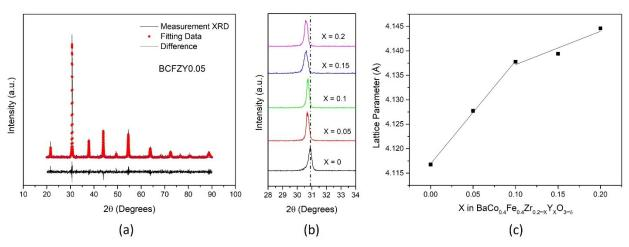
**Figure 1.** Structural data for (**a**) BCFZY0.05 with Rietveld refinement, (**b**) all compositions for (110) plane, and (**c**) lattice parameter calculated from XRD.
