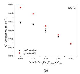
**Figure 7.** (a) The characteristic thickness,  $L_C$ , at 600 °C, calculated from ECR measurements for each BCFZY<sub>X</sub> composition. (b) Oxygen ion conductivity estimated using the Wagner equation with and without a correction for the characteristic thickness.
