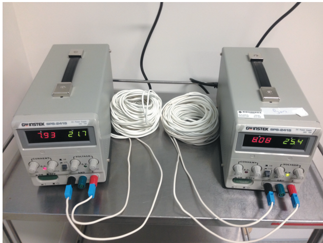
Figure 1: View of the 2 units of 24-V transformer and regulator and the heating cable. Several lengths of cable are available although in the present study we always used 2 sets of 17 meters of length.
