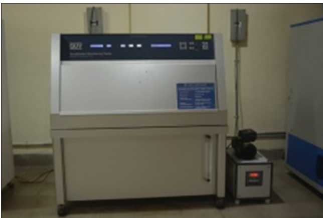
Figure 9: QUV accelerated weathering Tester (Q Labs, USA)
