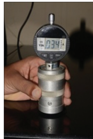
Figure 12: Shore A durometer readings noted
