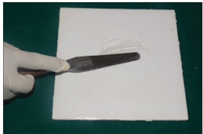
Figure 2: Base and catalyst mix for the nonpigmented room temperature vulcanizing group
