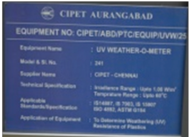
Figure 10: Accelerated aging protocol in accordance to IS 15907
