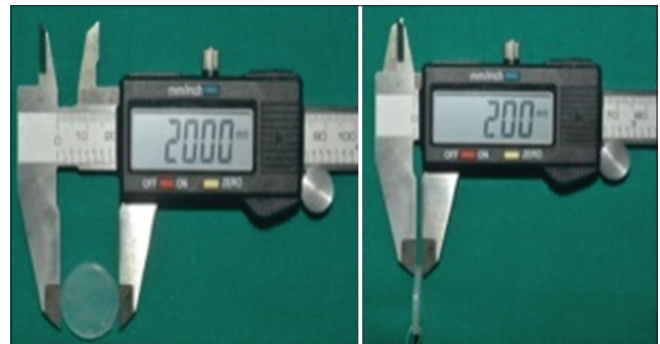
Figure 4: Nonpigmented room temperature vulcanizing silicone specimens of specified dimensions
