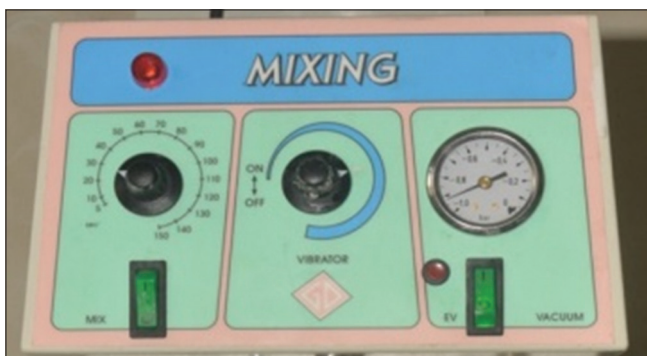
Figure 5: Vacuum deaeration at 0.9 bars for 5 minutes
