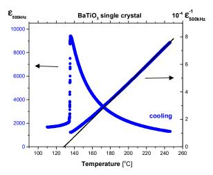
**Figure 1.** Temperature dependence of the real part of the complex permittivity and its inverse shown on the left and right ordinate, respectively, which was measured at the probe frequency of 500 kHz upon cooling. The solid line is the best-fitted result for the inverse dielectric constant in the paraelectric phase obtained by using the Curie–Weiss law (see the text).
