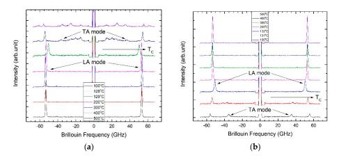
**Figure 2.** Temperature dependence of the Brillouin spectrum of BaTiO<sub>3</sub> measured at the backward scattering geometry upon (**a**) cooling and (**b**) heating. The phonon propagation direction was <100>. The LA and the TA mode indicate the longitudinal and the transverse acoustic mode, respectively. The ferroelectric phase transition temperature  $T_C$  is indicated by a horizontal arrow.
