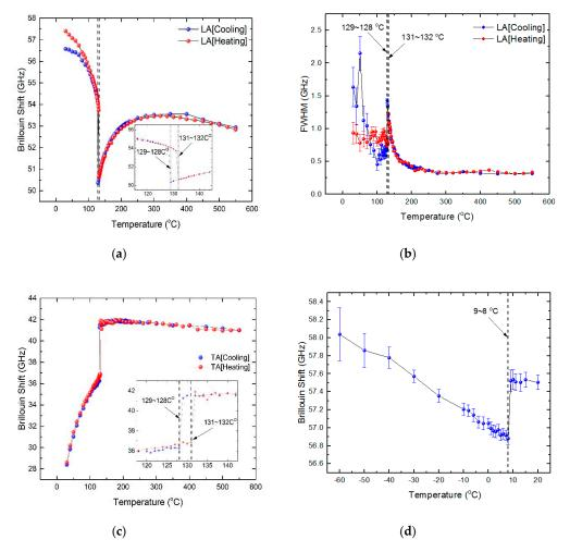
**Figure 3.** Temperature dependence of (**a**) the Brillouin shift of the LA mode, (**b**) the full width at half maximum (FWHM) of the LA mode, (**c**) the Brillouin shift of the TA mode, and (**d**) the Brillouin shift of the LA mode around the tetragonal–orthorhombic transition point. The two insets in (**a**,**c**) are the extended views of the data in the vicinity of  $T_C$ . The temperature ranges given in numbers denote the phase transition temperatures.
