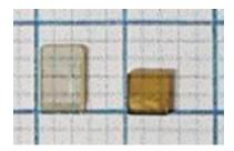
**Figure 7.** The left and the right single crystals were grown in terms of TSSG and SSCG method, respectively. The TSSG-grown BaTiO<sub>3</sub> single crystal was investigated in Reference [17].
