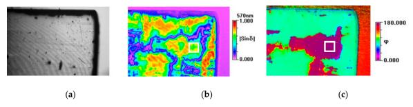
**Figure 5.** Maps of (a) the transmitted light intensity of 570 nm wavelength, (b) the  $|\sin \delta|$ , and (c) the angle φ measured for BaTiO<sub>3</sub> single crystal at 250 °C, far above  $T_C$ . The meaning of each symbol is described in the text. The rectangle visible in Figure (c) is the area of  $160 \times 100 \ \mu m^2$  for which the data shown in Figure 6a were calculated. Black points in (a) are the air pores visible on the crystal surface.
