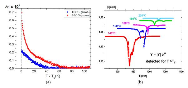
**Figure 6.** (a) Temperature dependence of the birefringence of both BaTiO<sub>3</sub> single crystals above T<sub>C</sub>. The data of the TSSG-grown BaTiO<sub>3</sub> was taken from Reference [17]. (b) Local minimum of the phase shift of the admittance accompanying piezoelectric resonances measured in the paraelectric phase for the virgin crystal by means of dynamic method and presented at several temperatures.
