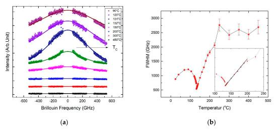
**Figure 4.** Temperature dependence of (a) the depolarized (VH) spectrum and (b) the FWHM of BaTiO<sub>3</sub> measured in a wider frequency range of  $\pm 540$  GHz ( $\pm 18$  cm<sup>-1</sup>). The inset shows the extended view of the FWHM near  $T_C$ . The solid line denotes the fitting result in terms of Equation (1).
