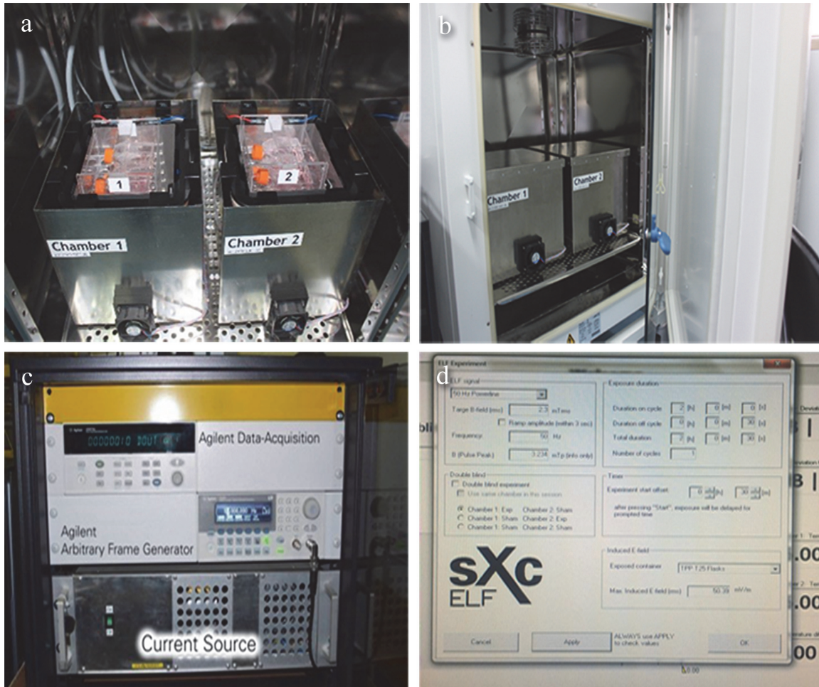
Fig 1. The PF-EMF exposure system. (a) mu-metal box; (b) incubator; (c) current source; (d) arbitrary function generator controlled by a computer.
