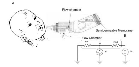
For the EP measurement, a rubber silicon tube can be placed on the outer surface of the nipple of a feeding bottle [27,29,32,34,48] (see Figure 5a). One end of the catheter (the extremity inside the mouth) is closed, while the other end is connected to a PT by means of a polyethylene catheter. This measuring system presents a limitation due to the rapid reaching of a plateau corresponding to the
