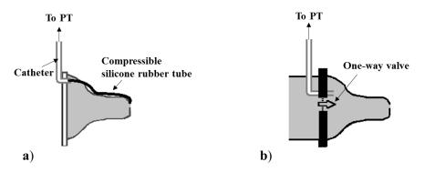
**Figure 6.** Sensing solutions for the measurement of the net pressure forcing the nutrient out of the nipple chamber. Two PTs are adopted to measure intranipple and intraoral pressure, and calculate the pressure gradient causing the nutrient to flow out.
