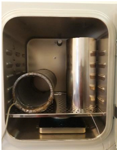
Fig. 5. Experimental setup to study long-term exposure to ELF-MFs (the exposure system on the left side and mu-metal cylinder on the right side)
