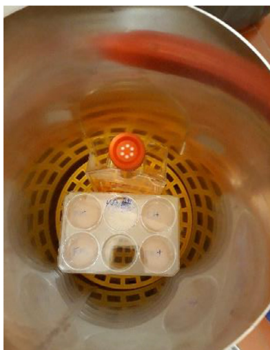
Fig. 6. View inside the mu-metal cylinder with the support (orange holder) to position the cells at the center of the cylinder
