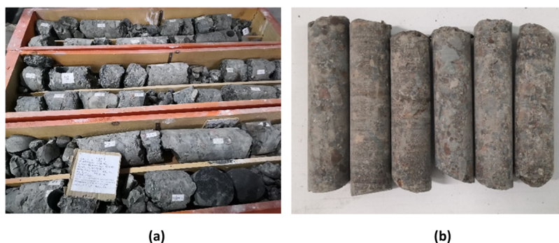
Figure 1. Reservoir rock samples from the Wuerhe formation ((a) 10-cm-diameter cores, (b) 2.54-cm-diameter cores).
