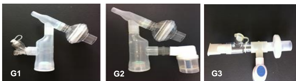
Figure 1. Nebulizer configurations used in this study. G1: mesh nebulizer with VHC, G2: jet nebulizer with VHC, and G3: jet nebulizer alone.
