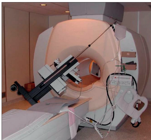
Figure 2. An example of “flying objects” hazards – regular infusion pump (MR Unsafe), presenting a hazard while used in MRI chamber, was pulled by static magnetic field of MRI magnet [ http://www.MRIsafety.com – with permission of Frank G. Shellock, Ph.D.] [5].
