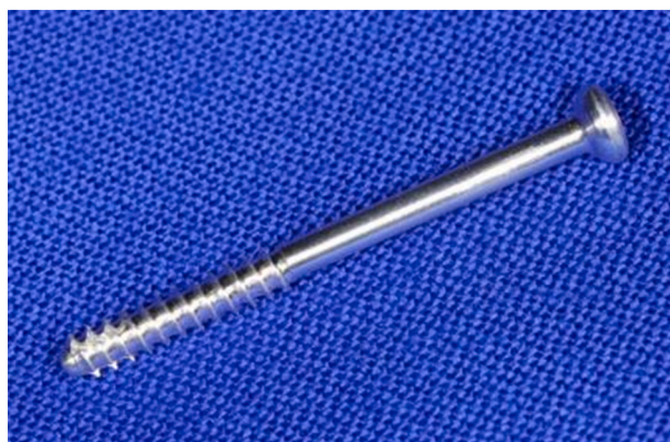
Fig. 1. External appearance of ZX00 screw with a length of 40 mm and a diameter of 3.5 mm, partly threaded at the distal part.
