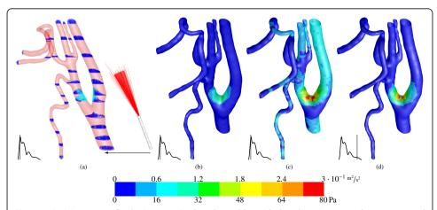
Figure 4 In (a) vectors of velocity magnitude coloured by turbulent kinetic energy k are presented (range above the colour bar). The catheter on the right is displaced from its origin in the CCA centre. The mean velocity at CCA inlet is  $0.38 \text{ ms}^{-1}$  and at cisplatin inlet  $7.66 \text{ ms}^{-1}$ . Figure (b) shows the related contour plot of k. Figure (c) and (d) are plots of wall shear stress in systole and diastole (range below the colour bar).
