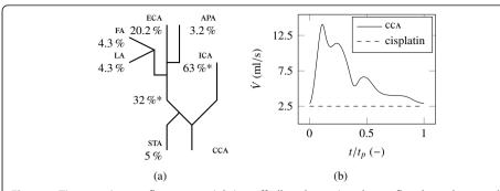
Figure 3 Time continuous flow rate weighting off all outlets using the outflow boundary condition in Figure (a). The asterisked values are the original time averaged data of [21]. The CCA flow rate inlet condition in Figure (b) is realized as a transient table with 200 equal distant timesteps (0.0047s timestep size). The cycle time  $t_0$  is 0.923s, which is equal to 65 heart beats per minute.
