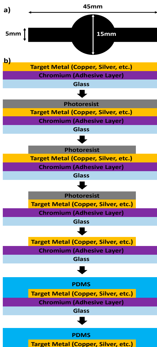
Figure 1. An illustration of chemical-free metal polydimethylsiloxane (PDMS) thermal bonding method. (a) A simple design for a mold to create a copper layer pattern. The mold was composed of a rectangular pattern size of 5 mm × 45 mm and a large circle at the center (diameter is 15 mm); (b) illustrations of the metal transfer process. Initially, metal layers were deposited on glass, firstly chromium (adhesive layer) then the target metal such as copper. The pattern of the target metal was fabricated by conventional photolithography and wet etching. Uncured PDMS was then poured on the metal surface. The curing conditions such as the PDMS mixing ratio, baking temperature and baking time was varied based on optimal adhesion parameters. After the PDMS was cured, the PDMS was peeled off of the transferred target metal layer.
