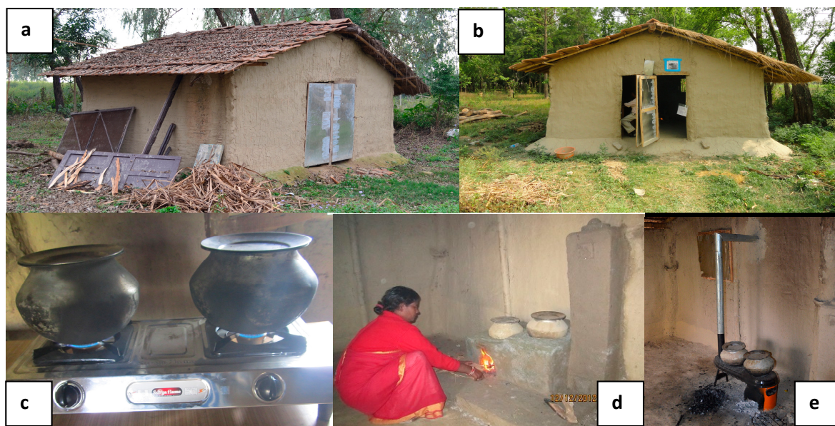
Figure 2. Study II photos of testing house and stoves used in water boiling test study in rural Nepal. (a) Single room test house (closed door), (b) single room test house (open door), (c) liquid propane gas stove (LPG), (d) alternative mud brick stove-II (AMBS-II), and (e) Envirofit G-series stove (representing MAES and NAES).
