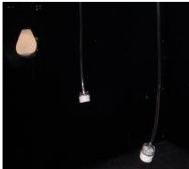
Figure 2 Diagram of the bioaerosol sampling cassette assembly (top), photograph of a cassette attached to a sampling pump (centre) and photograph of the cassettes in operation in the cough chamber (bottom).
