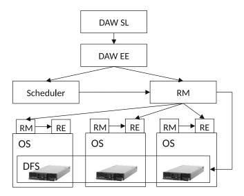
**Fig. 2** Components of a distributed DAW infrastructure (highly idealized). Abbreviations are explained in the text. For simplicity, the figure disregards many alternatives and extensions, such as virtualization, multi-core nodes, or network channels
