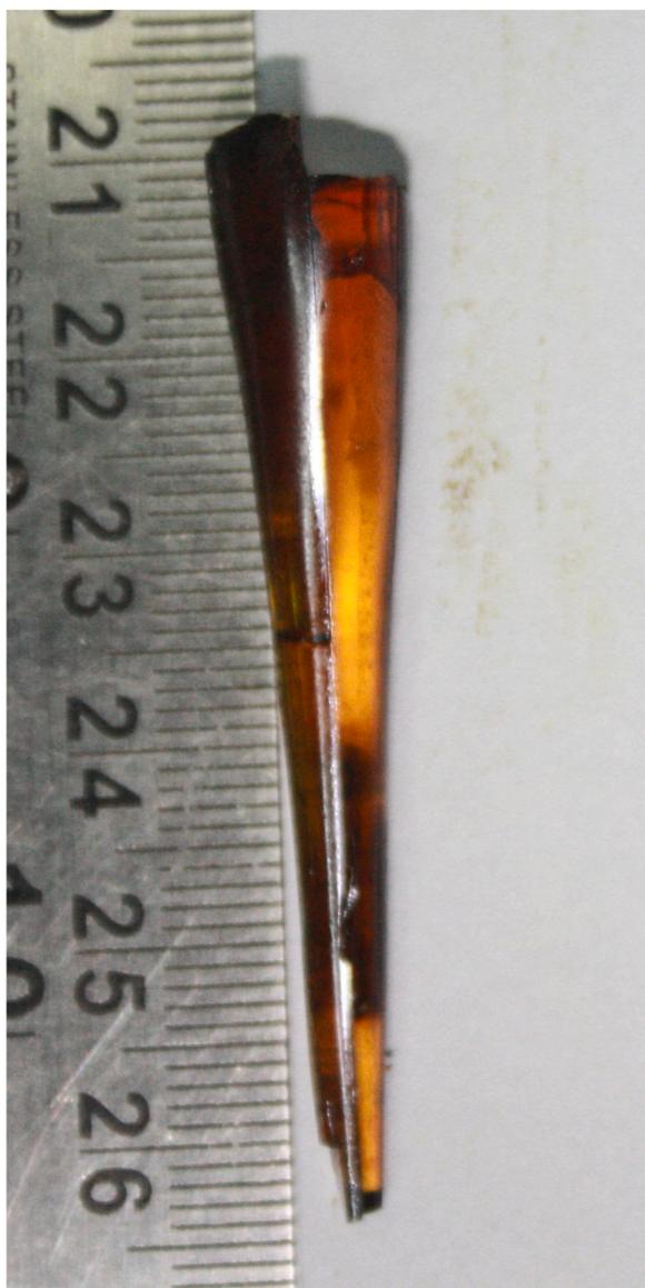
Fig. 6. The Bulk single crystal of 2-amino 4-methylpyridinium 4-nitrophenolate 4-nitrophenol grown by VBT.
