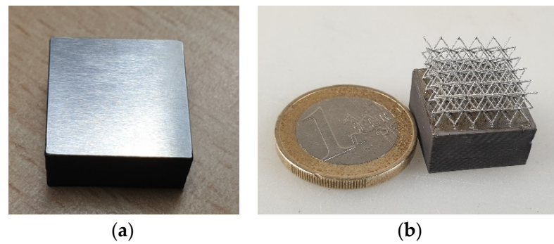
Figure 13. NiTi fabricated samples: (a) Substrate of 17 \times 17 \times 10 \text{ mm}^3 produced by FFF technology and (b) Hybrid structure including LPBF part (bcc lattice structure of 12 \times 12 \times 6 \text{ mm}^3 ) built on FFF part.
