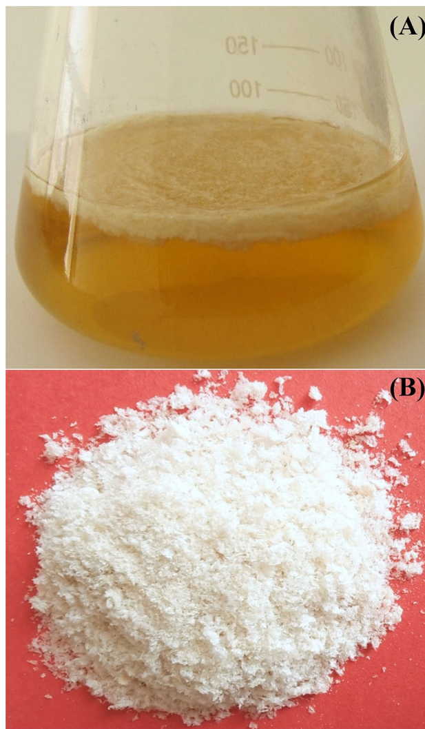
Figure 1. (A) Bacterial cellulose layer produced at the air–liquid interphase on medium no. 1; (B) Purified powder of the BNC.
