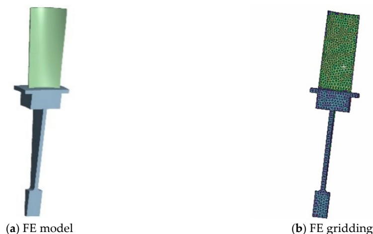
Figure 3. FE model and gridding of a turbine blisk.
