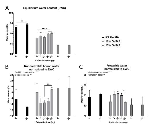
**Figure 11.** Water content and water types for GelMA hydrogels (5% to 15% gel fraction) crosslinked with 0, 3, 15, 30 or 90 µg cefazolin in PBS. Hydrogels were analyzed just after crosslinking. (**A**) Equilibrium water content (*EWC*) (%) (n = 5). (**B**) Non-freezable bound water ( $W_{nfb}$ ) (%) normalized to the *EWC* (n = 3). (**C**) Freezable water ( $W_f$ ) (%) normalized to the *EWC* (n = 3). Ns = non-significant; \* = p < 0.05; \*\* = p < 0.01; \*\*\* = p < 0.001; \*\*\* = p < 0.001.
