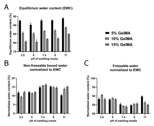
**Figure 7.** Water content and water types for GelMA hydrogels (5% to 15% gel fraction) crosslinked in water and swelled in media of different pH and fixed ionic strength of 150 mM. (**A**) Equilibrium water content (*EWC*, n = 5). (**B**) Non-freezable bound water ( $W_{nfb}$ ) normalized to the *EWC* (n = 3). (**C**) Freezable water ( $W_f$ ) normalized to the *EWC* (n = 3).
