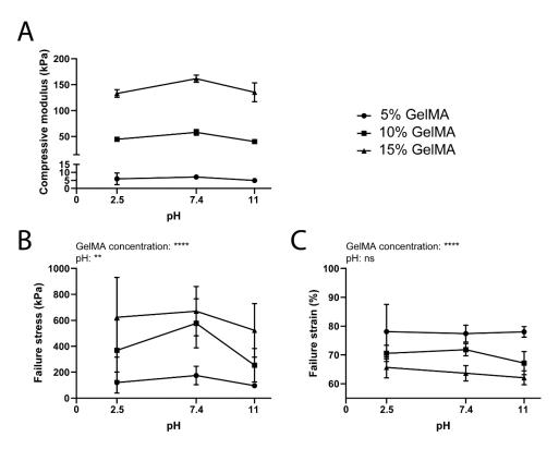
**Figure 9.** Mechanical properties for GelMA hydrogels (5% to 15% gel fraction) swelled at different pH. (**A**) Compressive modulus. (**B**) Failure stress. (**C**) Failure strain. Data are shown as means  $\pm$  standard deviation, n = 6-8. \*\* = p < 0.01; \*\*\*\* = p < 0.0001.
