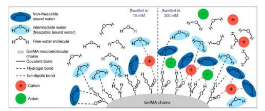
**Figure 6.** Graphic illustration of the proposed mechanism of water–GelMA interactions in GelMA hydrogels swelled at different ionic strengths.  $W_f$ ,  $W_{nfb}$  and free water molecules are presented with the same conventions as in Figure 3. On the right, the highest ionic strength of the swelling media reinforces the  $W_{nfb}$  fraction, more than for the lowest ion concentration on the left, due to increased number of ion–dipole bonds.
