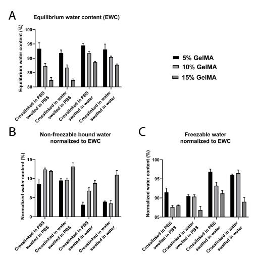
**Figure 2.** Water content and water types for GelMA hydrogels (5% to 15% gel fraction) crosslinked and swelled in different media. (**A**) Equilibrium water content (EWC, n = 5). (**B**) Non-freezable bound water ( $W_{nfb}$ ) normalized to the EWC (n = 3). (**C**) Freezable water ( $W_f$ ) normalized to the EWC (n = 3).
