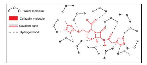
**Figure 12.** Graphic illustration cefazolin interaction with water molecules at pH 7.4. The polar hydrogen, nitrogen, sulfur, and oxygen atoms can form hydrogen bonds with water molecules.
