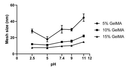
**Figure 8.** Mesh size for GelMA hydrogels (5% to 15%) crosslinked in water and swelled at different pH.
