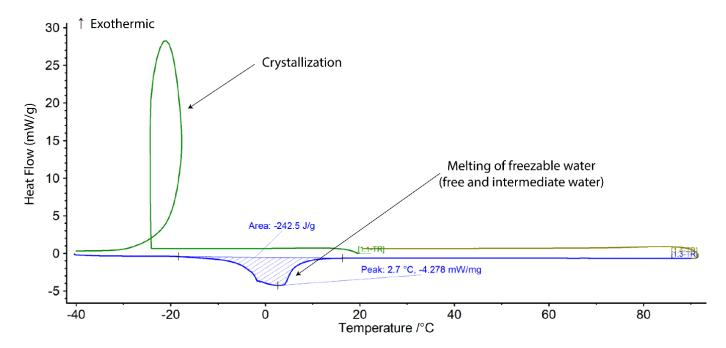
Figure 1. Differential scanning calorimetry (DSC) thermogram of 15% GelMA crosslinked in PBS and swelled in PBS.
