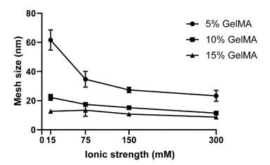
**Figure 5.** Mesh size for GelMA hydrogels (5% to 15%) crosslinked in water and swelled at different ionic strengths.
