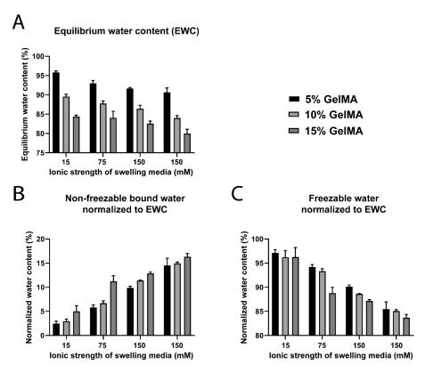
**Figure 4.** Water content and water types for GelMA hydrogels (5% to 15% gel fraction) crosslinked in water and swelled at different ionic strengths. (**A**) Equilibrium water content (EWC, n = 5). (**B**) Non-freezable bound water ( $W_{nfb}$ ) normalized to the EWC (n = 3). (**C**) Freezable water ( $W_f$ ) normalized to the EWC (n = 3).
