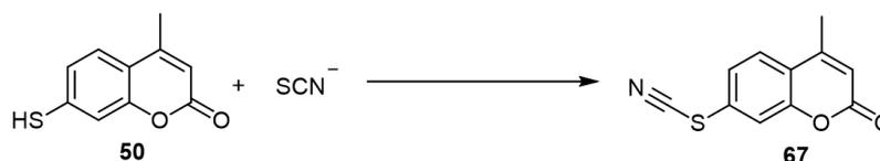
**Scheme 22.** Direct photocatalytic S–H Bond cyanation with green “CN” source. Reagents and conditions: Rose Bengal (1 mol%),  $CH_3CN$ , r.t., 12 h, white light (10 W), 52% yield.
