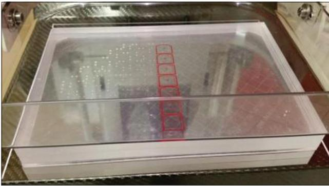
Figure 2: CDMAM phantom with 4 plates PMMA (photo: M. Biegala)
