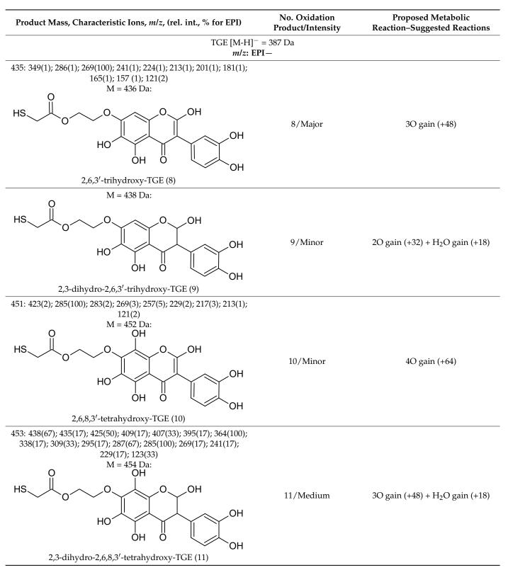
**Table 2.** Summary of proposed structures of main products of TGE formed after oxidation with 0.34 M  $H_2O_2$ , 0 V.
