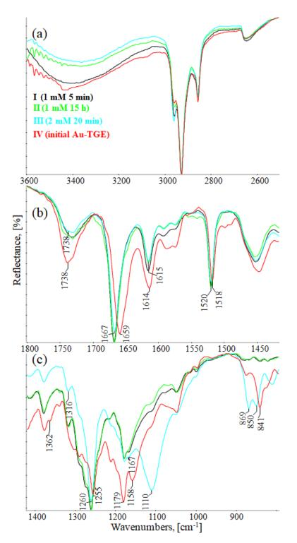
**Figure 10.** IR-ATR spectra of Au-TGE before and after oxidation with  $H_2O_2$ , (**a**) from 3600 to 2500 cm<sup>-1</sup>; (**b**) from 1800 to 1425 cm<sup>-1</sup>; (**c**) from 1400 to 800 cm<sup>-1</sup>.
